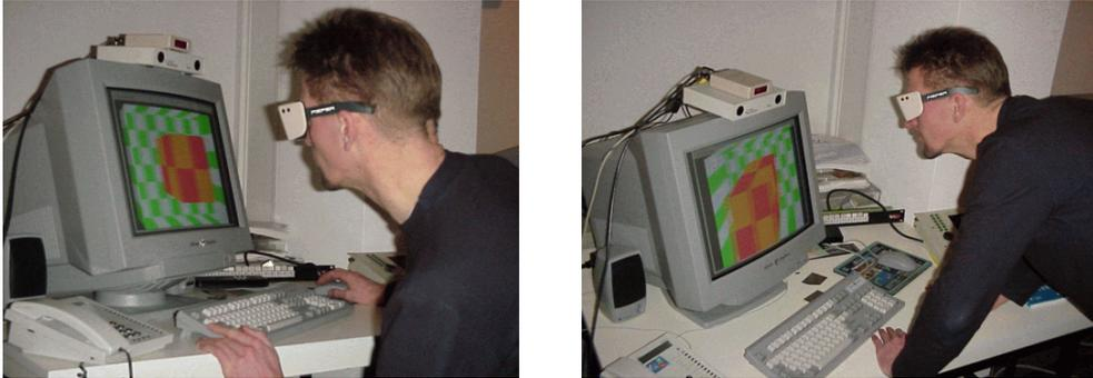
**Figure 5.9** The test environment. The head tracker is on top of the display, the infrared transmitter for the LCD shutter glasses is on top of the tracker.
